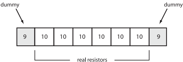
Figure 5–10. Dummy devices take the hit of the over-etching, protecting our real devices in the center.
