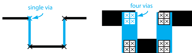
Figure 8–3. Thicker wire allows additional vias between metals.
