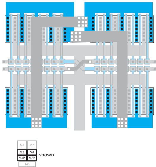
Figure CSI-42. Cross-quad area finished. Device outputs are connected in Metal Two with plenty of vias and wire width to allow good current flow.
