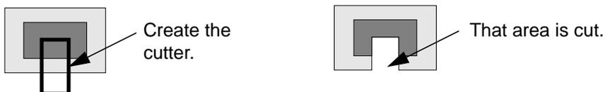
If you create a polygon cutter, you must double-click to complete the polygon cutter and the chop.
