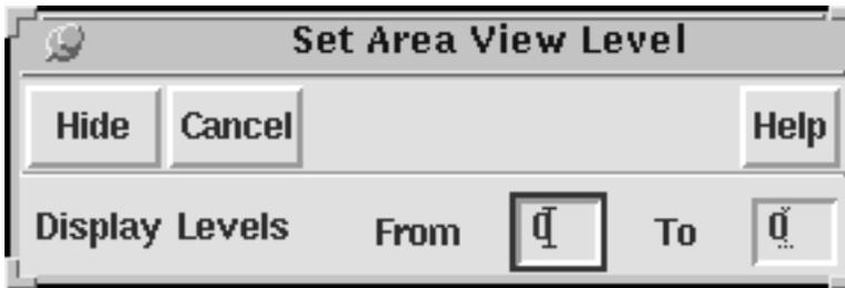
**Display Levels** specifies the first (*From*) and last (*To*) levels in the design hierarchy that can be seen in detail. The hierarchy levels are numbered 0 to 32. Shapes in the current cellview are at level 0, shapes in the masters of instances inside of it are level 1, and so forth.
